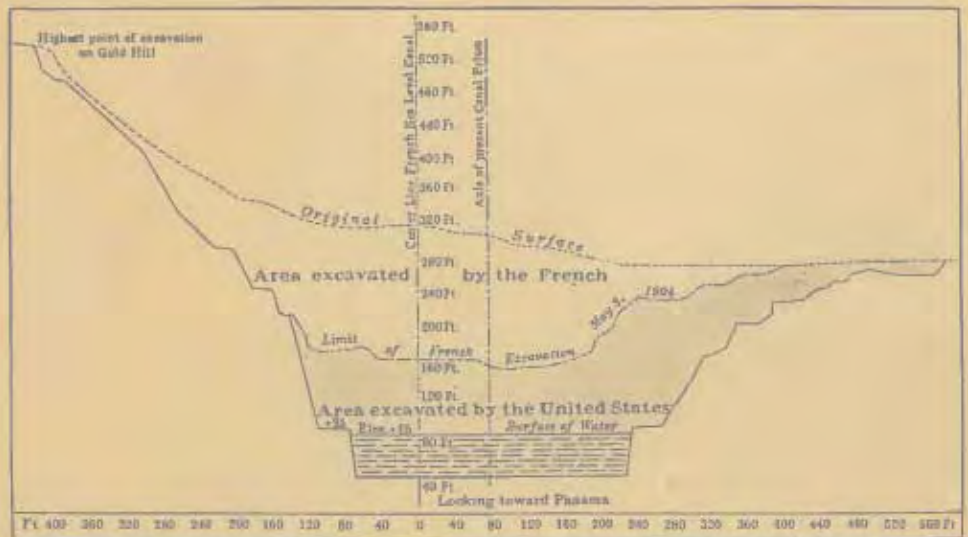
DIAGRAM OF COMPARATIVE EXCAVATIONS BY THE FRENCH AND AMERICANS IN CULEBRA CUT
